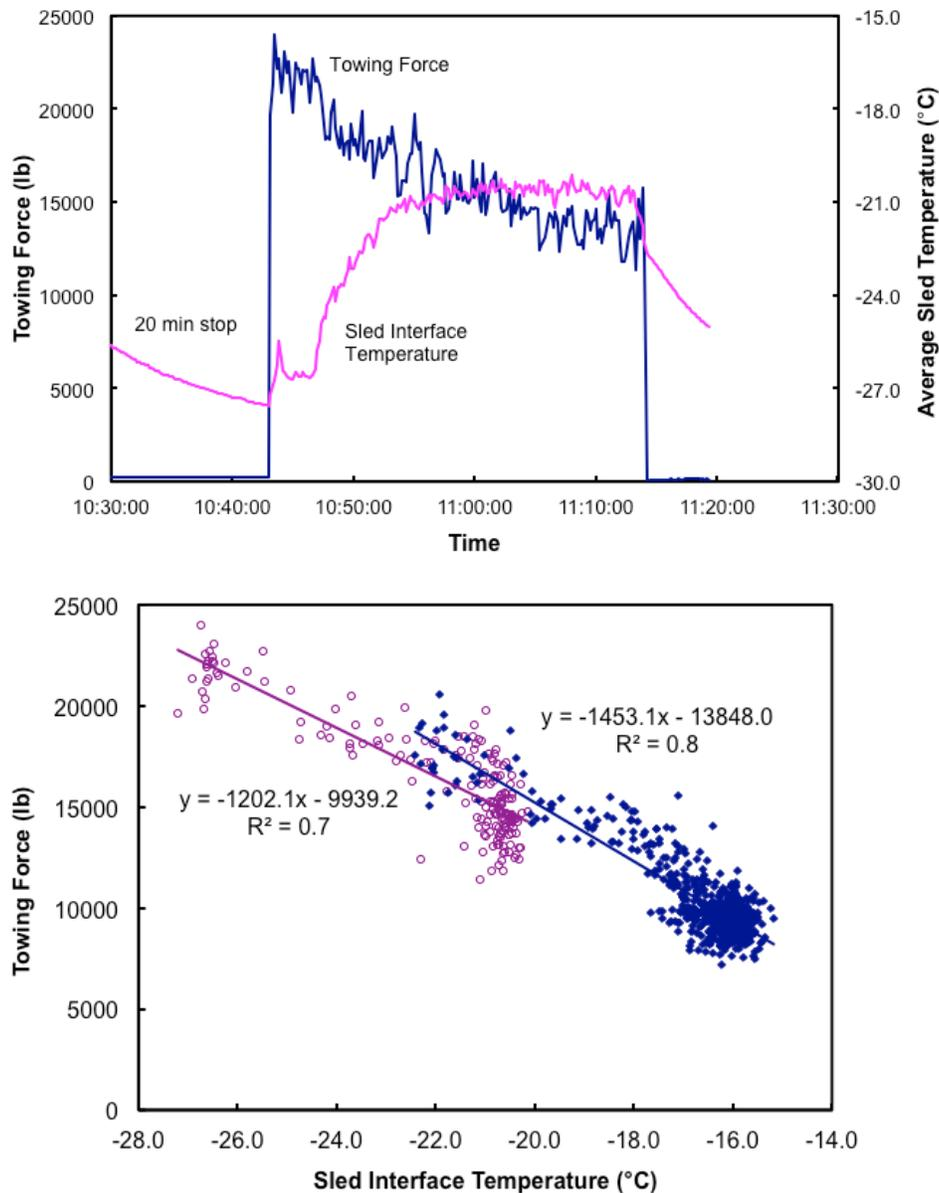
From experiments conducted en route during GrIT10, we obtained more comprehensive measurements to investigate methods to enhance warming of the sled–snow interface (Lever 2011a). We instrumented two bladder sleds with thermocouples and used separate load pins between the sleds
