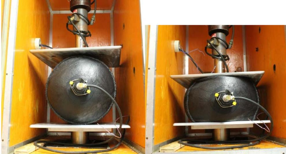
Figure 23. Two-layer construction of a FFF sample pontoon (*upper*) mimicked that of the larger pontoons supplied for tube-in-pouch ARCS (*lower*): an impermeable liner (*clear*) resided within a tough, woven outer shell (*black*). The pouch material in 2011–12 was two-tone with a gray exterior and a tan interior.
