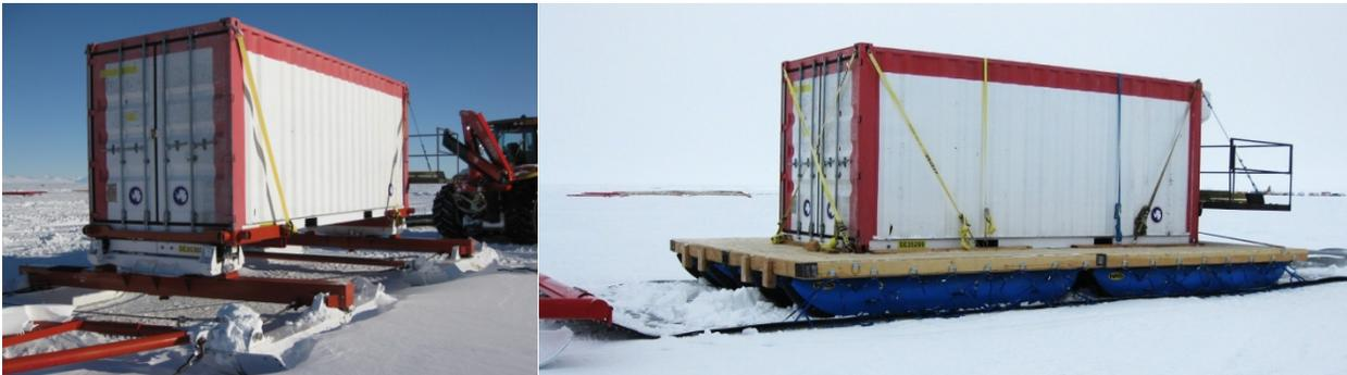
GrIT11 had more time to procure two revised ARCS that included custom-made pontoons and higher strength–weight ratio decks. Tare weight dropped to 5000 lb, and pre-departure tests with 23,000 lb of payload yielded a payload efficiency of  $W_p/T \approx 6$ . Importantly, both ARCS completed the 1460-mile Thule–Summit round trip with no pontoon failures although high air-leakage rates and snow intrusion between the pontoons demanded another round of design revisions.
