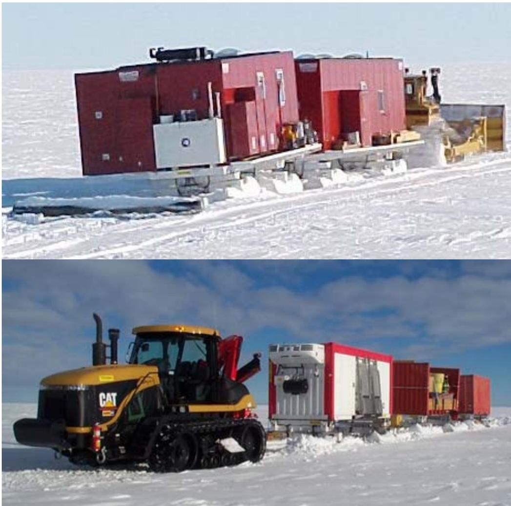
Figure 15. The flat rack and tool shed supported on modified ISO kits during SPoT04-05. Longer benches placed the skis outside of the tractor ruts, but the sleds retained their high tare weight.
