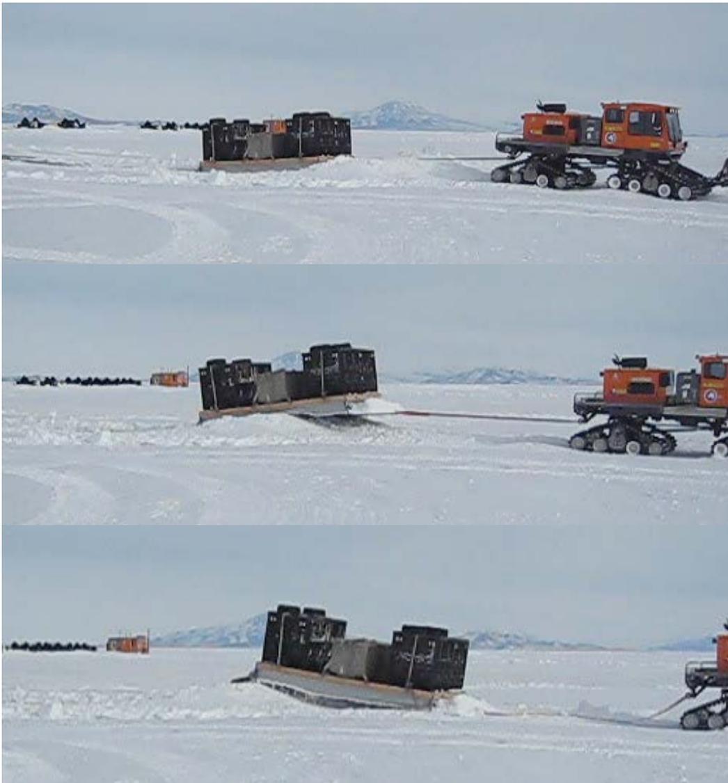
The PIG11-12 ARCS performed very well throughout the field season, based on feedback from PIG crew. The sleds completed approximately 1700 miles of travel, much of it over soft snow and large sastrugi. The ARCS rode well and had no problems with snow intrusion, air leakage, or pouch material failure. PIG12-13 used the same ARCS with similarly successful results.
