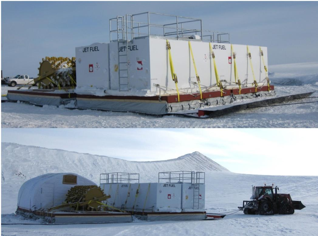
GrIT12 crew reported good stability and ride quality of the ARCS along with no pontoon leaks. The only minor issue arose early: two pouches developed tears at their corners where they were bolted to the HMW-PE sheets (Figure 27). The crew installed diagonal straps (see Figure 29) to prevent further tearing, and the ARCS successfully completed their round trips with no further issues. GrIT12 delivered a total of 66,000 lb of cargo to Summit on ARCS.
