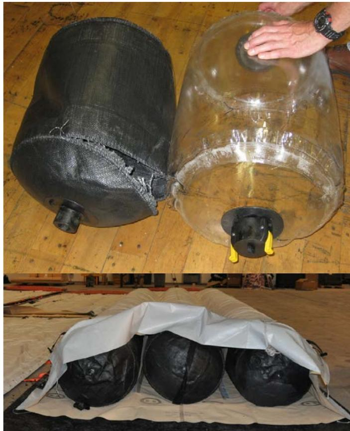
SPoT chose not to construct and deploy its ARCS for 2011–12 owing to last-minute season-mission changes. However, the PIG traverse crew assembled and deployed four smaller ARCS, each consisting of 8 ft wide × 16 ft long wood-framed decks supported by four 18 in. diameter × 16 ft long pontoons in a single, four-sleeve pouch (Figure 24). These ARCS were sized to fit inside an LC130 aircraft and designed to carry 10,000 lb of payload each (Lever 2011c).
