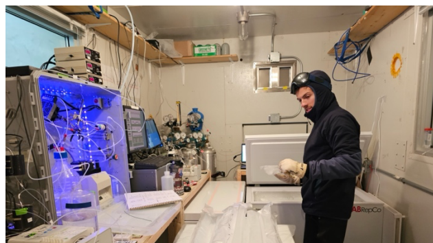
Figure 3. Our team set up a warm lab inside the Bally Building to analyze ice cores for carbon monoxide, methane, black carbon, and other chemical species. Here, Ben Riddell-Young is organizing ice cores for analysis.
